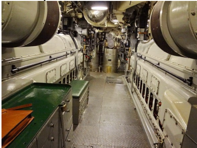
Two of the four Fairbanks Morse Model 38D-1/8 10 cylinder engines on the submarine.
